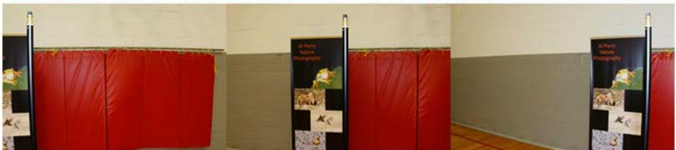
With lens rotating about its optical center, parallax is eliminated as black pole remains fixed relative to background
