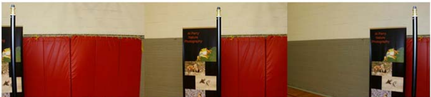
With lens not rotating about its optical center, parallax is seen as black pole in foreground moves relative to background
