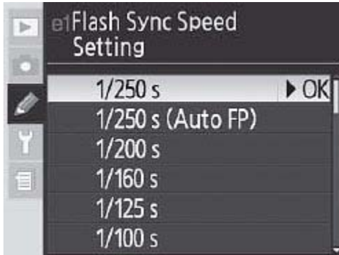
Nikon D2x Menu Set Custom Setting e1 to 1/250 s (Auto FP) to enable High Sync mode.
